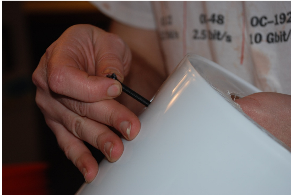
Figure 14 - Push one end of the bungee cord through the 1/4" hole in the side of the bucket. Repeat for the other piece of bungee on the other side of the bucket.
