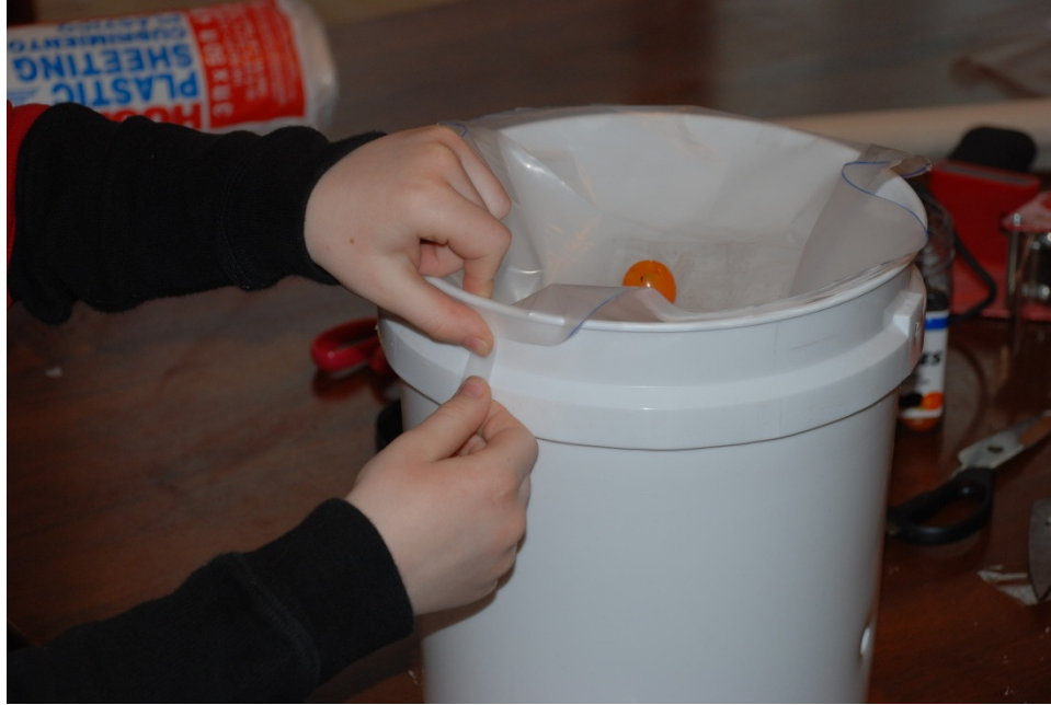
Figure 12 - Using Scotch tape, we very roughly attached the plastic circle to the bucket. The bungee cord side goes in and the orange plastic ball side goes out. The plastic needs to be attached so that the outer circle of the plastic is approximately at the edge of the bucket. Since the diameter of the plastic circle is larger than the bucket, this results in some bunching up of the plastic. The goal of the tape here is not to necessarily attach the plastic well, but just enough until the next step.
