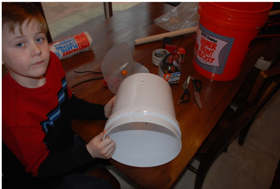
Figure 11 - Cut two small holes in the side of the bucket near the bottom. We used a 1/4" drill bit and drilled them 2" from the bottom. The holes need to be on opposite sides of the bucket for the bungee cord to go through. If you don't have a 1/4" drill bit, scissors or a utility knife will do. Just don't cut the holes too large.
