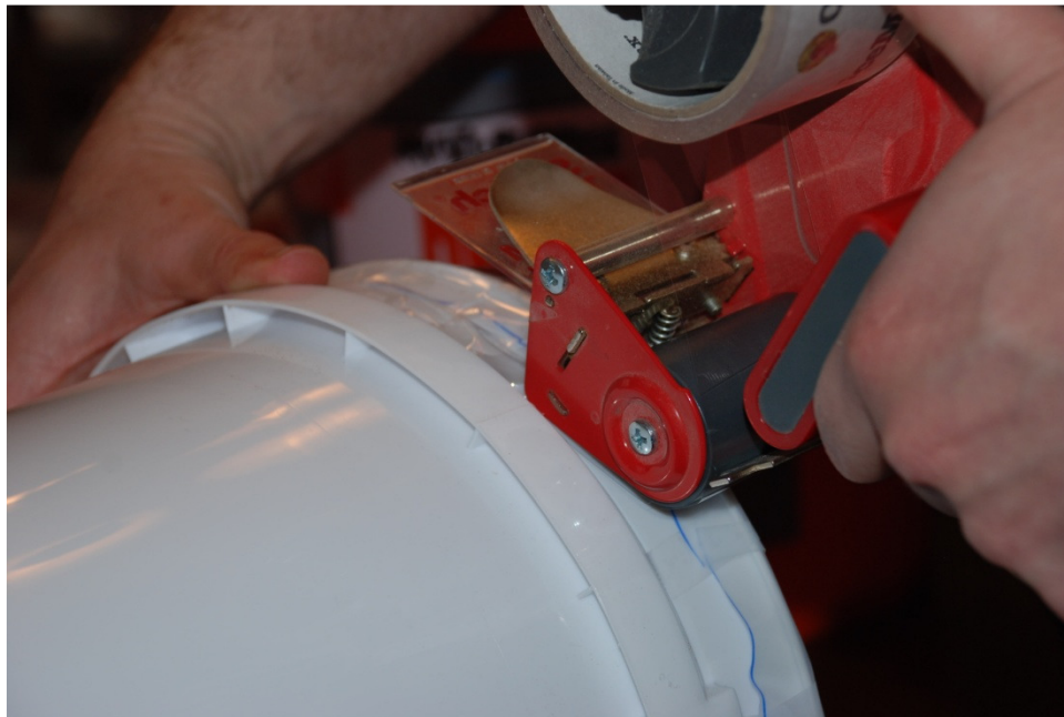
Figure 13 - Seal the plastic circle to the bucket with packing tape. We ran the tape about \frac{2}{3} over the bucket, and \frac{1}{3} hanging over the edge. After applying the tape, the \frac{1}{3} that was left hanging over the edge was pressed over into the plastic sheet. This helps seal the plastic sheet and better secures it to the bucket.
