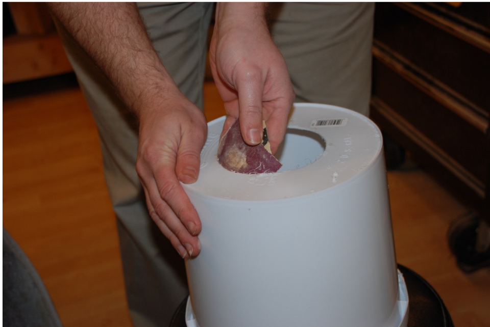
Figure 3 - We removed any sharp edges with 120 grit sandpaper.
