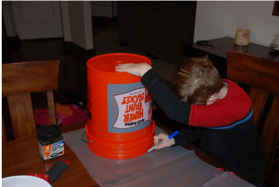
Figure 4 - Trace a circle in the 4 mil plastic sheeting. The "Homer Paint Bucket" was the perfect size. Yet another use for this amazing item.
